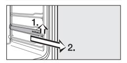
■ Lift the FlexiClip runner up at the front and pull it out along the rail.
